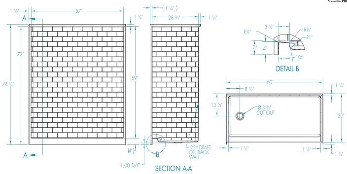
FEATURES Dimensional Tolerance ± 36". Dimensions needed for site preparation should be measured from the unit. Aquatic assumes no responsibility for preparatory work.
