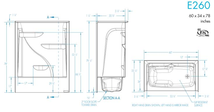
FEATURES lbs Dimensional Tolerance ± 3/8". Dimensions needed for site preparation should be measured from the unit. Aquatic assumes no responsibility for preparatory work.
