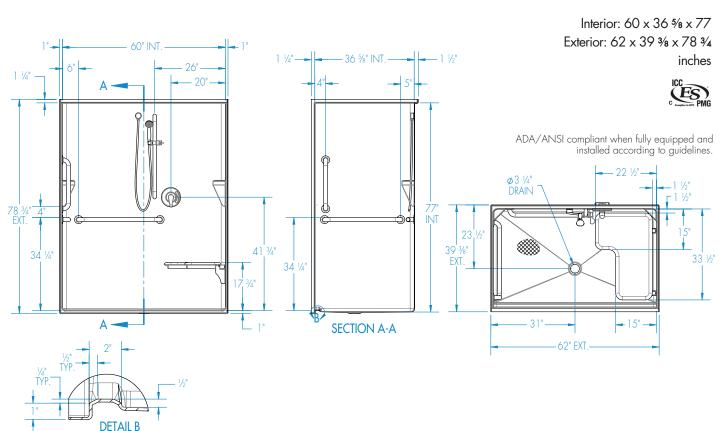
FEATURES Dimensional Tolerance ± 36". Dimensions needed for site preparation should be measured from the unit. Aquatic assumes no responsibility for preparatory work.
