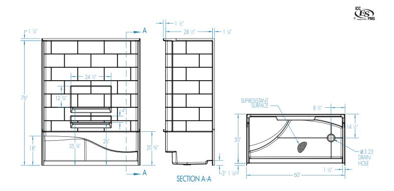
FEATURES Ibs Dimensional Tolerance ± 36". Dimensions needed for site preparation should be measured from the unit. Aquatic assumes no responsibility for preparatory work.
