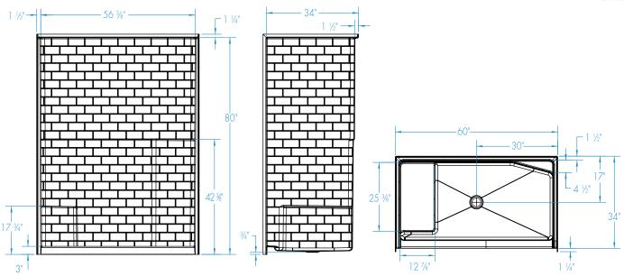
FEATURES Dimensional Tolerance ± %". Dimensions needed for site preparation should be measured from the unit. Aquatic assumes no responsibility for preparatory work.
