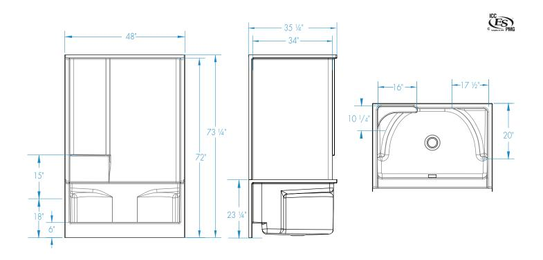
FEATURES Ibs Dimensional Tolerance ± 36". Dimensions needed for site preparation should be measured from the unit. Aquatic assumes no responsibility for preparatory work.
