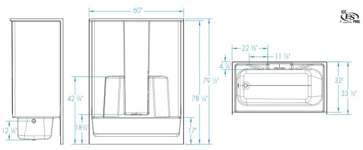
FEATURES lbs Dimensional Tolerance ± %". Dimensions needed for site preparation should be measured from the unit. Aquatic assumes no responsibility for preparatory work.
