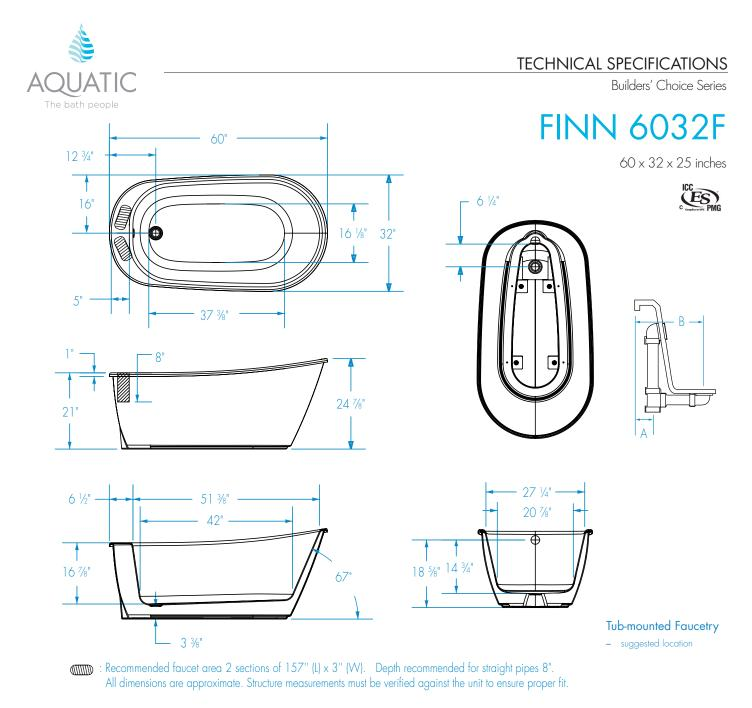
FEATURES Dimensional Tolerance ± 3/8". Dimensions needed for site preparation should be measured from the unit. Manufacturer assumes no responsibility for preparatory work.
