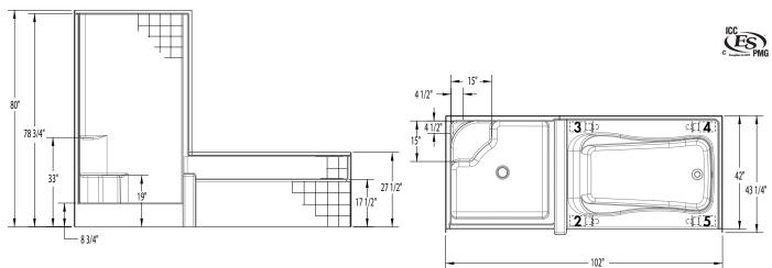
FEATURES Dimensional Tolerance ± %". Dimensions needed for site preparation should be measured from the unit. Aquatic assumes no responsibility for preparatory work.
