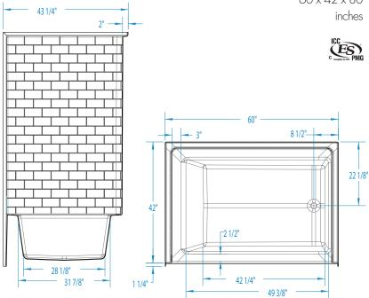
FEATURES Ibs Dimensional Tolerance ± %". Dimensions needed for site preparation should be measured from the unit. Aquatic assumes no responsibility for preparatory work.
