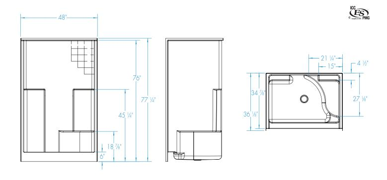
FEATURES Ibs Dimensional Tolerance ± %". Dimensions needed for site preparation should be measured from the unit. Aquatic assumes no responsibility for preparatory work.
