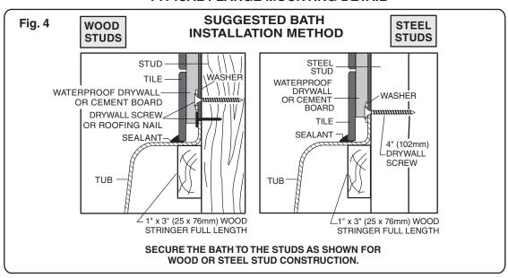
**C.)** Any finish material such as tile or wallboard must be self-supporting if it contacts the deck of the bath. Flooring will be butted against the bottom of the tub apron, also holding the tub in place.
