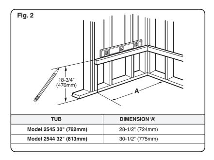
**D.)** Install drain components to the bath following the manufacturer's instructions. See the roughing-in drawing for suggested opening size and location dimensions.
