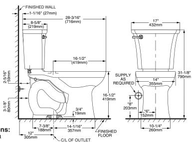
THIS TOILET IS DESIGNED TO ROUGH-IN AT A MINIMUM DIMENSION OF 305MM (12") FROM FINISHED WALL TO C/L OF OUTLET. SUPPLY NOT INCLUDED WITH FIXTURE AND MUST BE ORDERED SEPARATELY. \* DIMENSION SHOWN FOR LOCATION OF SUPPLY IS SUGGESTED.
