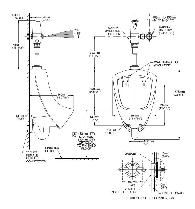
PROVIDE SUITABLE REINFORCEMENT FOR ALL WALL SUPPORTS.
