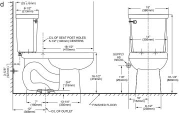
THIS COMBINATION IS DESIGNED TO ROUGH-IN AT A MINIMUM DIMENSION OF 305MM (12") FROM FINISHED WALL TO C/L OF OUTLET. \* DIMENSION SHOWN FOR LOCATION OF SUPPLY IS SUGGESTED. SUPPLY NOT INCLUDED WITH FIXTURE AND MUST BE ORDERED SEPARATELY.
