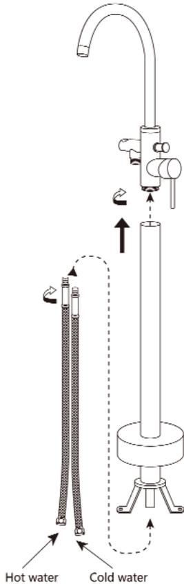
3 Feed Flexible Hoses (4) through Faucet Body Tube (8) and thread securely on to faucet connections.
