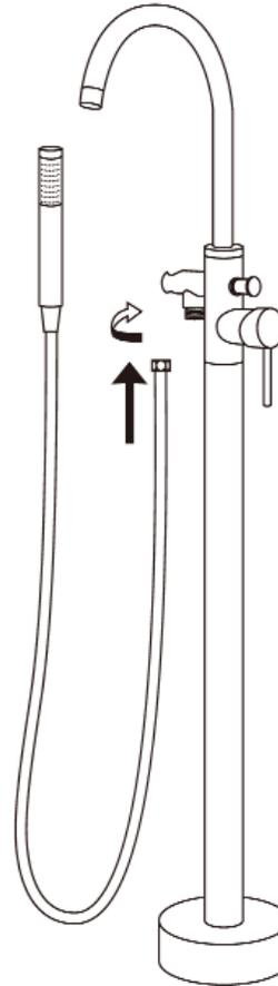
6. Connect the Handshower Hose (6) to both the Handshower and Faucet Body (2). Turn on water to test connections.
