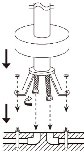
5. Tighten the Mounting Base (5) to the floor. Connect the Flexible Hoses (4) to the hot and cold water supplies. Hot and cold water lines will rough in just above the finished floor. Exact height to ber determined on site.
