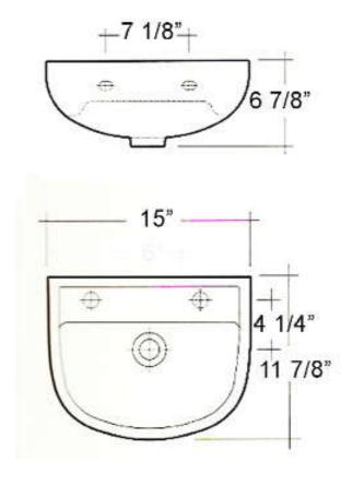
Dimensions of fixture are nominal and may vary within the range of tolerances established by ANSI Standard A112.19.2.2013 Dimensions and specifications subject to change without notice.
