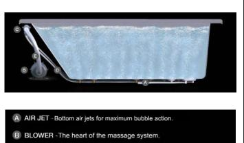
C MANIFOLD - Double back flow security prevention device.
