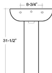
Dimensions of fixture are nominal and may vary within the range of tolerances established by ASME Standard A112.19.2-2008. Dimensions and specifications subject to change without notice.
