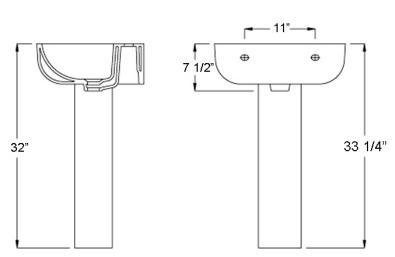
Dimensions of fixture are nominal and may vary within the range of tolerances established by ASME Standard A112.19.2-2008. Dimensions and specifications subject to change without notice.
