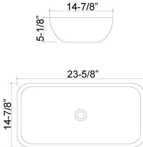
Dimensions of fixture are nominal and may vary within the range of tolerances established by AMSE Standard A112.19.2.2013 Dimensions and specifications subject to change without notice.
