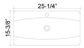
Dimensions of fixture are nominal and may vary within the range of tolerances established by AMSE Standard A112.19.2.2013 Dimensions and specifications subject to change without notice.
