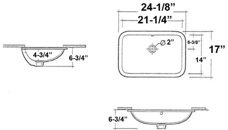
Dimensions of fixture are nominal and may vary within the range of tolerances established by ASMEI Standard A112.19.2. Dimensions and specifications subject to change without notice.
