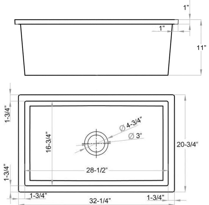
Dimensions of fixture are nominal and may vary within the range of tolerances established by ANSI Standard A112.19.9. Dimensions and specifications subject to change without notice.
