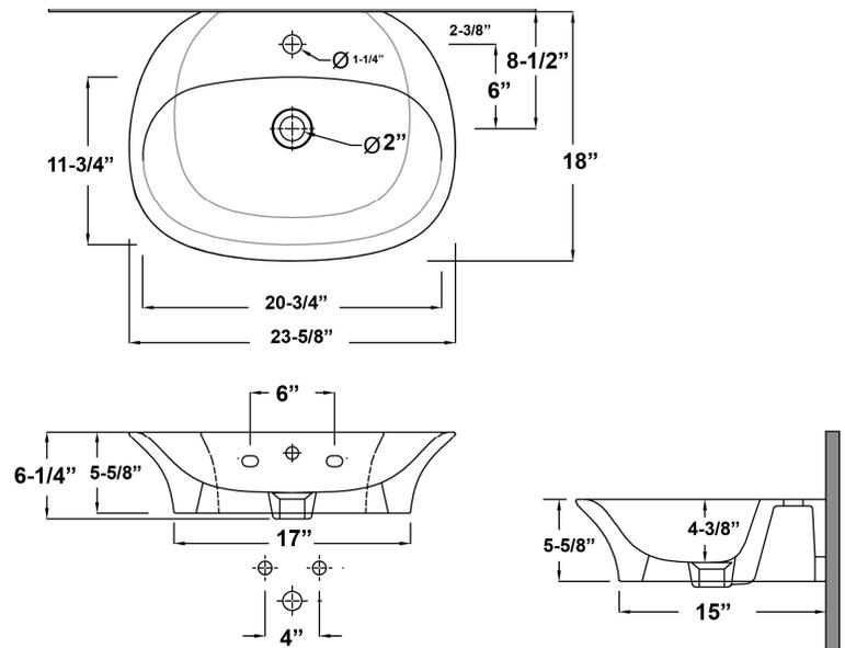
Dimensions of fixture are nominal and may vary within the range of tolerances established by ASME Standard A112.19.2.2018. Dimensions and specifications subject to change without notice.
