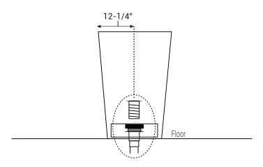
Thread the PVC drain fitting onto the waste flange. We recommend using a small amount of clear silicone on the threads of the PVC drain fitting to act as a thread sealant. Tighten until it seats, plus one quarter turn.
