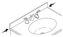
USE SILICONIZED ACRYLIC CAULK TO SECURE TO THE WALL
