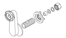
3. Attach the diverter lever (C) onto the diverter valve (D) and tighten the diverter screw.
