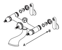
2. Thread the tapered ends of the nipples into the swivel mounts on the outside of the tub.
