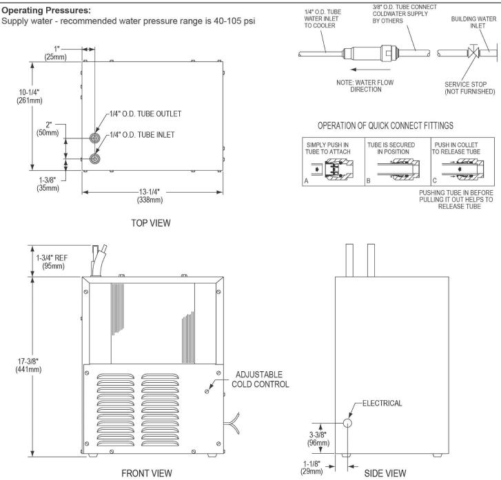
NOTE: When mounting unit in an open area, to ensure proper ventilation, maintain a 4" (102mm) clearance from cabinet louvers on each side of chiller. When mounting unit in a cavity or behind a wall, maintain minimum space of 4" (102mm) on each side, 4" (102mm) on the top and a depth of 12" (305mm).
