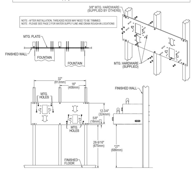
\*ADA REQUIREMENT NOTE - AFTER INSTALLATION, THREADED RODS MAY NEED TO BE TRIMMED
