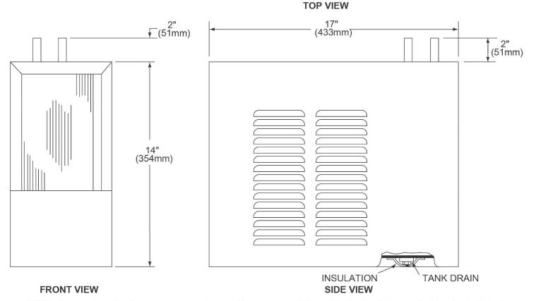
NOTE: It is important to insure proper ventilation. If this remote chiller is physically placed against barrier or in enclosure of any kind, 4" (102mm) air space must be allowed on all sides.
