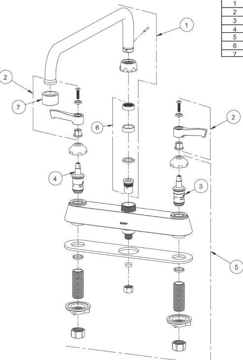
DESCRIPTION ITEM IND. PART A55399 1 Spout Handle, 4" 45919C 45923C **Right Cold Cartridge** Left Hot Cartridge 45924C 45914C Body 98554C **Backflow Kit** 2.2 GPM VR Aerator LK734
