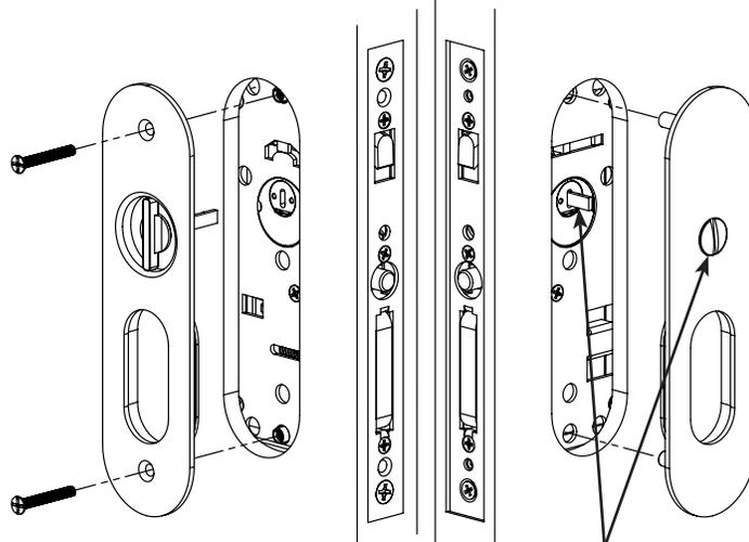
Align Passage/Privacy button with Thumb-turn spindle and secure trim plates to door.
