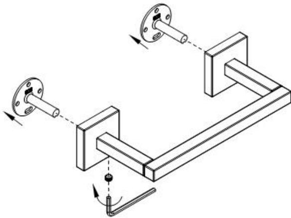
② ALIGN MOUNTING BRACKETS AND MARK LOCATION
