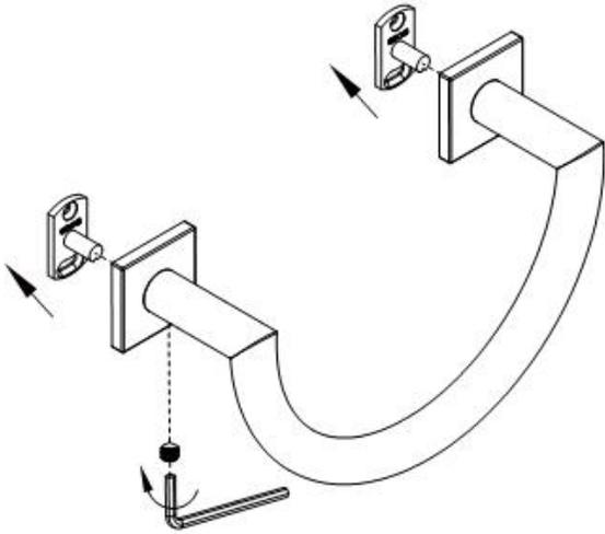
② ALIGN MOUNTING BRACKETS AND MARK LOCATION
