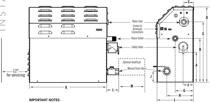
Provide a minimum of (12) inches at both ends and top of the steam generator or as required for servicing. Alternately, provide unions as required to facilitate installation and disconnection of the steam generator.
