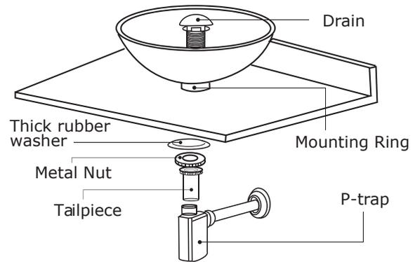
**Step 2 : Drain assembly picture**
