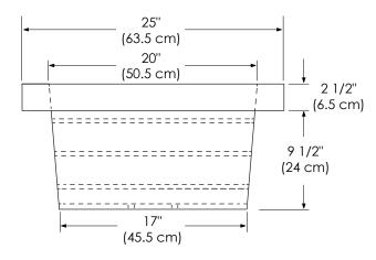
By IAPMO, ceramic lavatory warpage is defective only if warpage of flat slab out of horizontal plane exceeds 6.3 mm/m (0.25 in/ft) on all sizes OR warpage on back of lavatories that are attached to the wall exceeds 3 mm (0.13 in).
