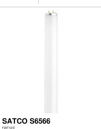
General Status Active Watts 20 Shape T12 Base Medium Bi Pin G13 ANSI Base Nominal Length 24 CCT (Kelvin) 6500 Temperature Daylight CRI 76 Lumens 1075 Beam Spread 360 Hours Rated 9000 Lamp Type Linear Technology Fluorescent Electrical **Operating Temperature Ballast Dependent** Physical MOL 23.78 MOD 1.5 Additional Information Warranty Avg. Rated Hour Limited Compliance Energy Star No CEC Status Lawful for sale in California **RoHS** Compliant Yes
