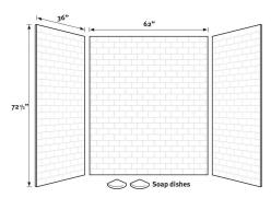
Designed to fit base areas 36" deep or smaller x 62" wide x 72-1/2" high or smaller (914 mm x 1575 mm x 1829 mm)
