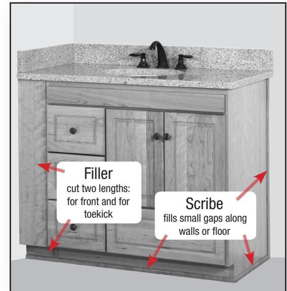
Cut Filler or Scribe to length and secure in place with adhesive or fasteners of your choice.
