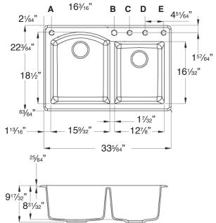
IMPORTANT: Circle Letter(s) above to indicate location(s) for faucet hole drillings (there is a 4" spread between hole locations B,C,D. There is a 163/16" spread between hole locations A and B and a 451/64" spread between D and E).
