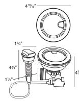
Turn the remote knob to open and close drain. Water drains easily when cover is in place. Cover flips up with easy touch. Polypropylene housing. Fits standard 3½" opening. 1¾" hole required in countertop for remote installation. Remote cable 25½" L.
