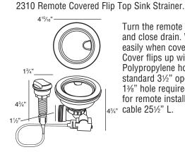
Turn the remote knob to open and close drain. Water drains easily when cover is in place. Cover flips up with easy touch. Polypropylene housing. Fits standard 31/2" opening. 1%" hole required in countertop for remote installation. Remote cable 251/2" L.
