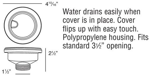
Water drains easily when cover is in place. Cover flips up with easy touch. Polypropylene housing. Fits standard 3<sup>1</sup>/<sub>2</sub>" opening.
