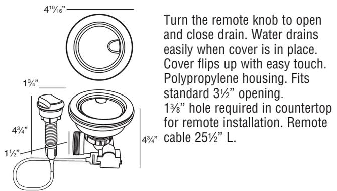
Turn the remote knob to open and close drain. Water drains easily when cover is in place. Cover flips up with easy touch. Polypropylene housing. Fits standard 3<sup>1</sup>/<sub>2</sub>" opening. 1<sup>3</sup>/<sub>8</sub>" hole required in countertop for remote installation. Remote cable 25<sup>1</sup>/<sub>2</sub>" L.
