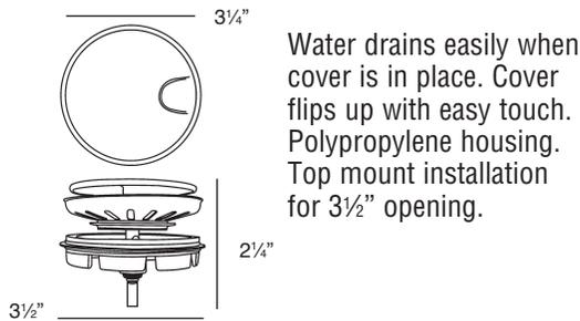
Water drains easily when cover is in place. Cover flips up with easy touch. Polypropylene housing. Top mount installation for 3<sup>1</sup>/<sub>2</sub>" opening.
