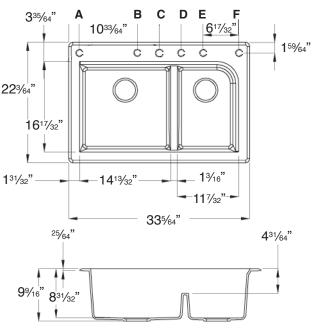
IMPORTANT: Circle Letter(s) above to indicate location(s) for faucet hole drillings (there is a 4" spread between hole locations B,C,D,E. There is a 10<sup>33</sup>/<sub>64</sub>" spread between hole locations A and B and 6<sup>17</sup>/<sub>32</sub>" between E and F).
