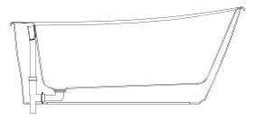
Standard drainpipe and overflow compatible with end-drain freestanding bathtub models: W2AX6032FTO.
