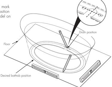
Place the bathtub in the previously marked position. Verify that the bathtub is completely leveled. Use the leveling legs if needed. Remove the bathtub.
