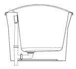
Standard drainpipe and overflow compatible with center drain freestanding bathtub model: W1AX6032FTO, W1AX6636FTO, W4AX6032FTO, W4AX6036FTO.
